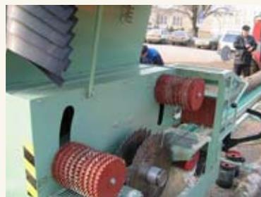
*Driven in-feed and out-feed rollers for sawing over a single arbor. Blades are easily changed from twin edger to multi-rip pattern*
