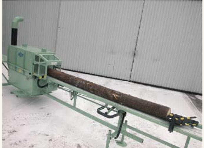
*The Kara PPS500 cuts logs 70 - 220 mm in diameter and 1.5 - 4m in length*
